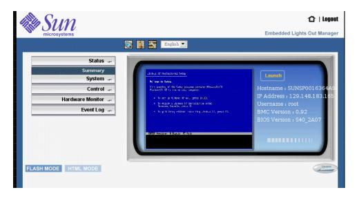
FIGURE 2-3 Initial Embedded LOM Screen
